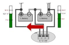
The second battery in the series has a voltage that is 0.3 V higher than the first battery in the series.
