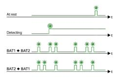
The system shows charge compensation on the LED display as a flashing code. The flashing code is composed of two parts:
